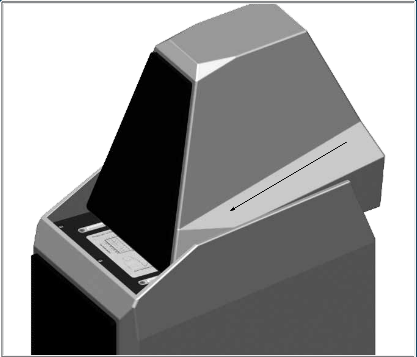
FIGURE 5 – SLIDE THE UPPER MIDRANGE/TWEETER MODULE'S FRONT SPIKES ALONG THE GUIDES IN THE TOP OF THE WOOFER MODULE, KEEPING THE REAR OF THE UPPER MIDRANGE/TWEETER MODULE ELEVATED TO AVOID SCRATCHING THE WOOFER MODULE.
